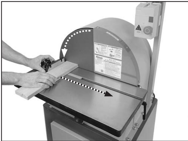
Figure 11. Example of X-axis sanding.
